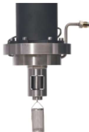
Sorption and density measurement with a magnetic suspension balance (sample basket and titanium sinker)
